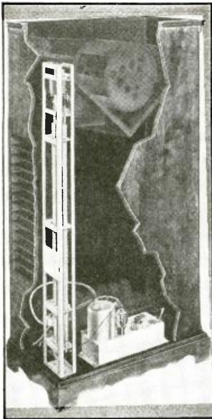
Cutaway view of the Hammond tone cabinet showing the shape and location of the new reverberation control unit. (See details in drawing, Fig. 1.)
